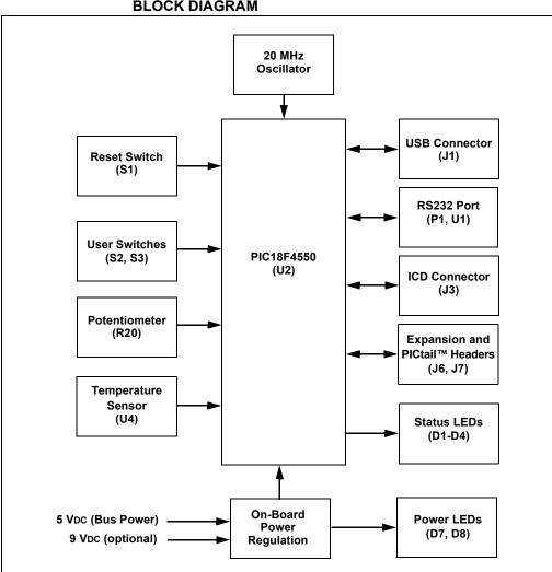
FIGURE A-1: PICDEM<sup>™</sup> FS USB DEMONSTRATION BOARD FUNCTIONAL BLOCK DIAGRAM
