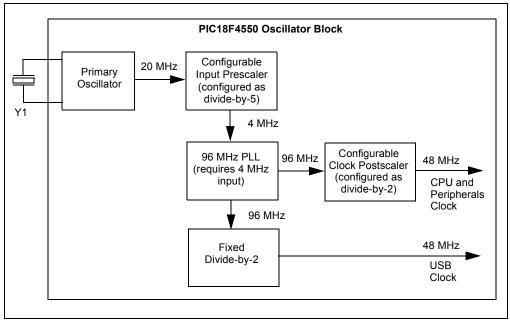
FIGURE 1-2: PIC18F4550 CLOCK SETUP FOR PICDEM™ FS USB
